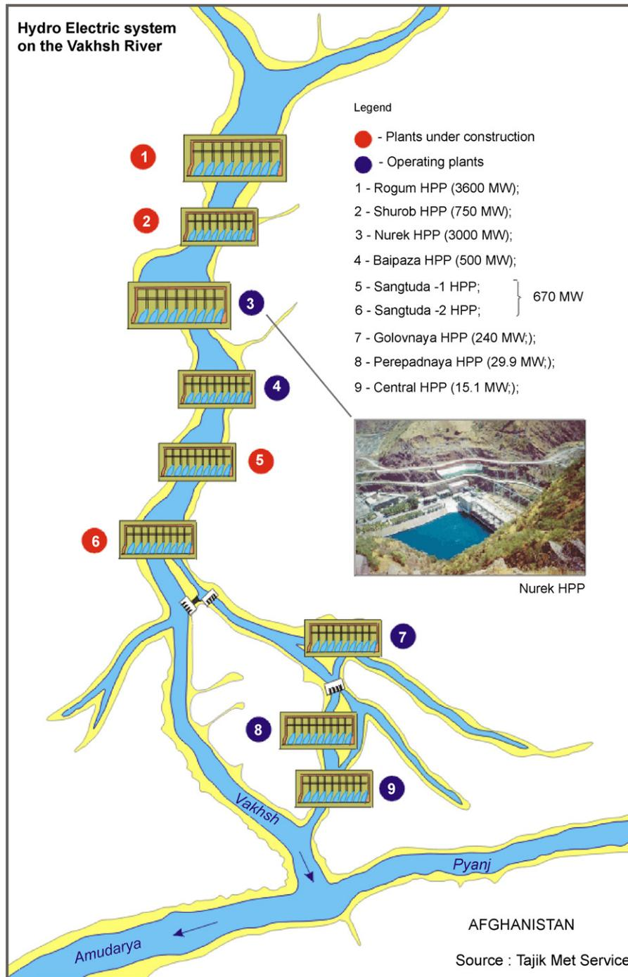
Fig. 6. Current and planned infrastructure in the Vakhsh Basin. Source: World Bank, 2004, p. 23.
