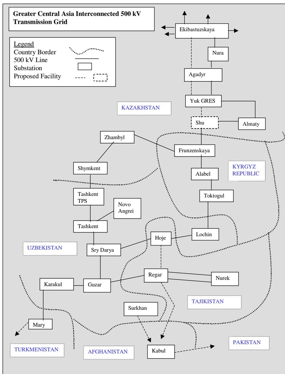
Fig. 5. Transmission grid in Central Asia. *Source: USAID report, 2004.*
